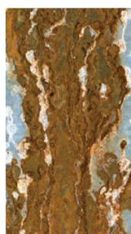
Hot-dip galvanisation 20 µm after 6 weeks
