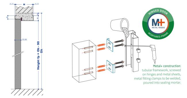
REMARKS: The principle of these section drawings is valid for almost all our swing doors. The standard thickness of the doorleaf is 72 mm. The fireproof doors EI1 60 have a thickness of 82 mm! For doors with exceptional performance features such as fireproof doors EI1 120 and HCM 120/EI2 240, two-way doors, burglary resistance doors RC4 and RC5, ... other section drawings are available, see: www.heinen-doors.com.
